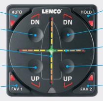
TO OVERRIDE AUTOMATIC SETTINGS (AUTO, FAV 1, FAV 2, OR HOLD) AND MANUALLY CONTROL THE TRIM TABS, SIMPLY PRESS ANY OF THE UP OR DN BUTTONS. AT THIS POINT, ALL AUTOMATIC BOAT CONTROL DECISIONS STOP AND YOU ASSUME FULL MANUAL CONTROL OF THE TRIM TABS.
